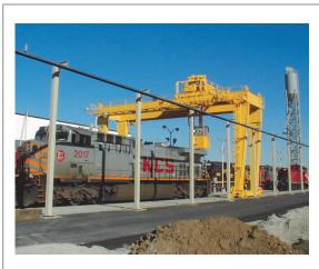
Sand Gantry Cranes are the safest method available for sanding locomotives on multiple tracks. Operators ride in a cab on the crane which eliminates the danger of climbing on the locomotive. The sand storage silos are designed to suit site requirements.
