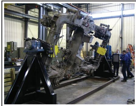
Macton's rotator system turns the vehicle on its central axis at a convenient working height to facilitate disassembly, inspection and maintenance. It is also able to be mounted on rails and moved around the shop
