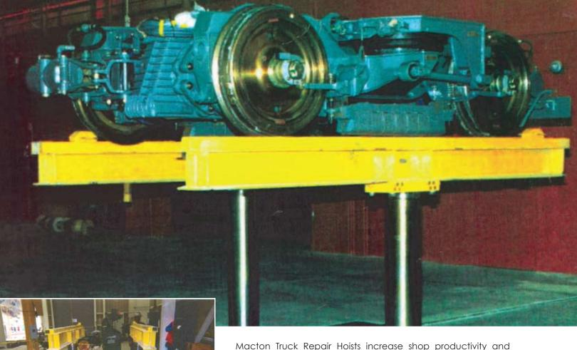
Macton Truck Repair Hoists increase shop productivity and safety by allowing shop personnel to perform maintenance, repair and inspection of rail vehicles that are elevated at a convenient height above the shop floor.
