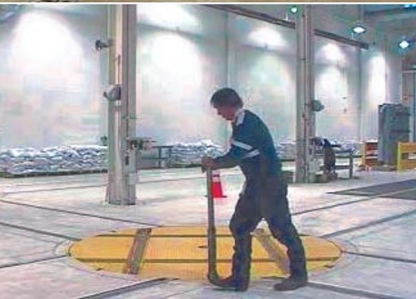
Macton Truck Turntables are used for transferring vehicle rail truck assemblies from a service track to other tracks within a maintenance facility.
